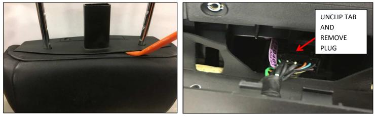
**3.** Remove the 2 x screws and lift up surround from the bottom and pull the top of the screen out, it can take a little force as it can be quite tight.
