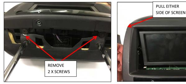
**4.** Remove the 2 screws from either side and turn screen upside down and unclip the plastic surround at the 4 points and then remove the harnesses from the top of the screen.
